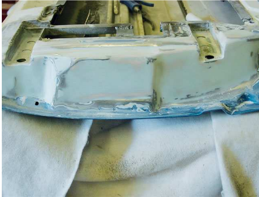
Smooth the front side of the door after all of the metal fabrication
