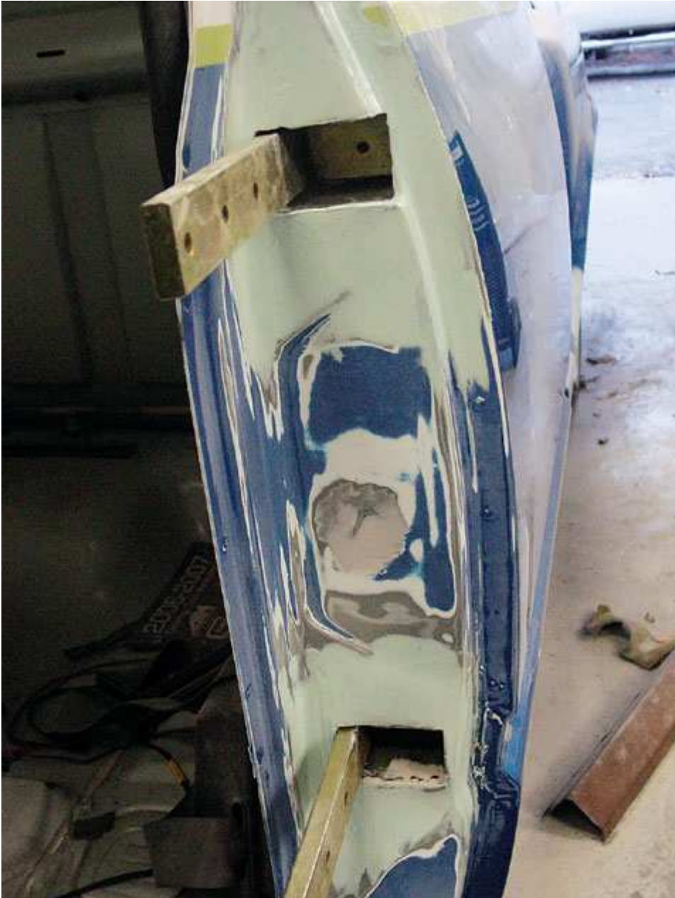
While doing the fender bodywork, smooth all of the hinge areas.
